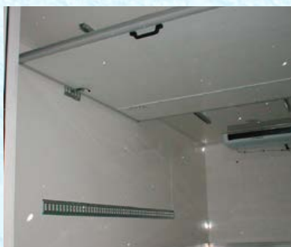
Transversal partition wall movable and tiltable
