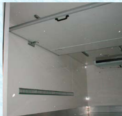
Transversal partition wall movable and tiltable
