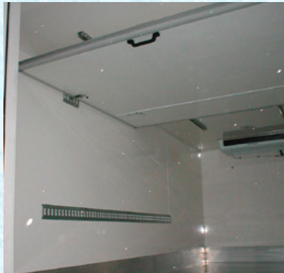
Transversal partition wall movable and tiltable
