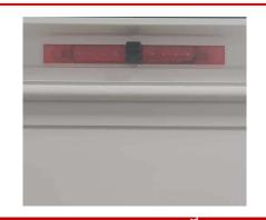
Reverse camera integrated in 3<sup>rd</sup> brake light
